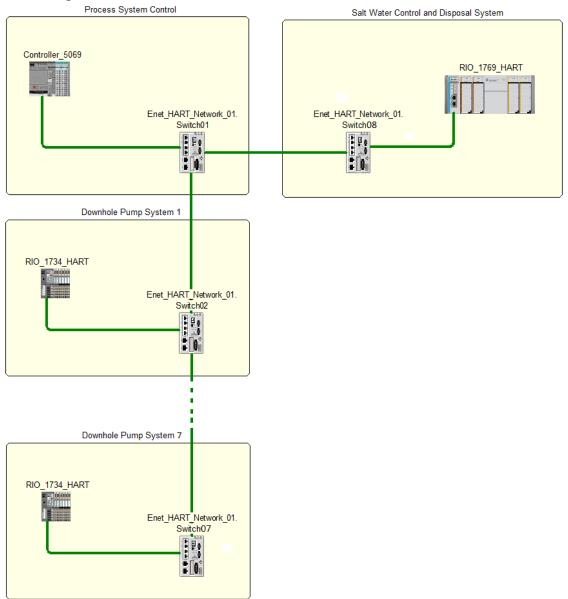
A process control system may have one system produced by one manufacturer, and multiple systems produced by another manufacturer, each using their own normal type of IO to integrate into the Process Control System. In this illustration there are 3 Rockwell platforms integrated together – the 5069, the 1734 and the 1769 platforms.
