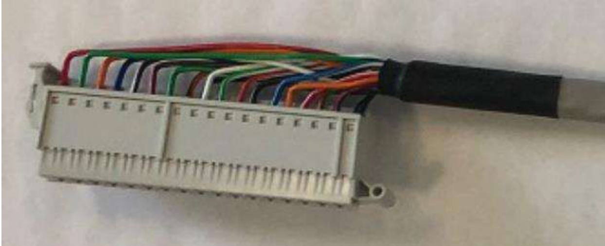
Figure 6. One of Two Conversion Module 18-Pin Connectors on the 5069 Side
