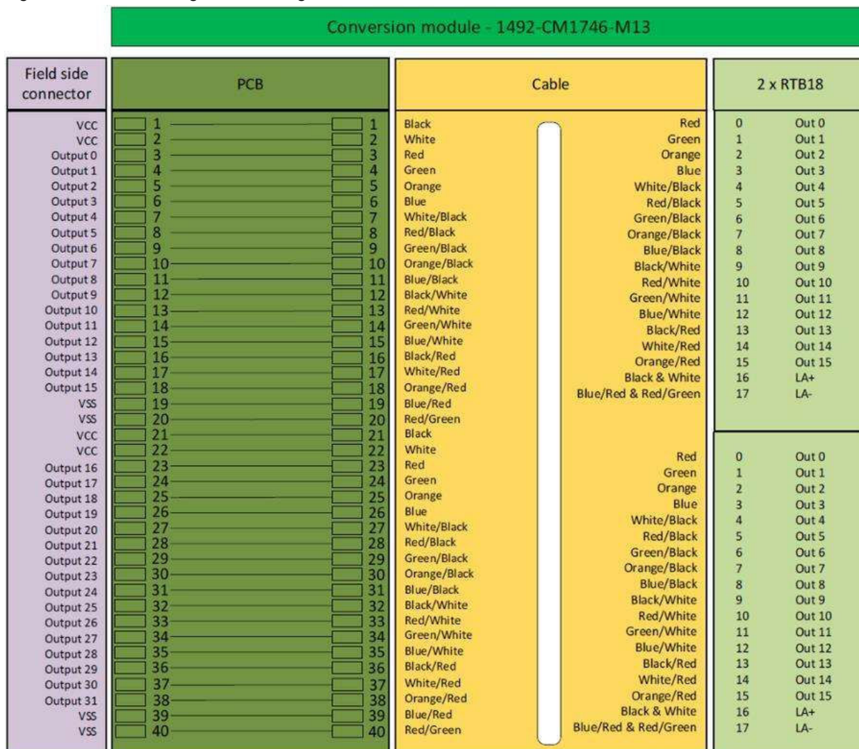
Figure 4. Rockwell Diagram Showing Connection Flow for the Conversion Module 1492-CM1746-M13
