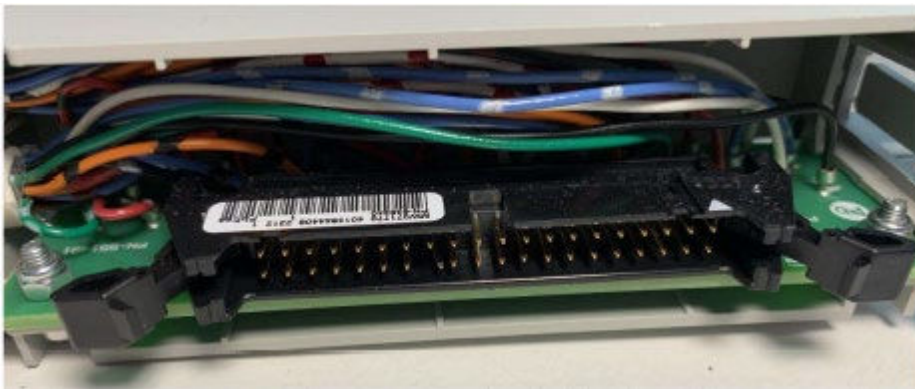
Figure 5A. Conversion Module 40-Pin Field Connector on the 1746 Side
