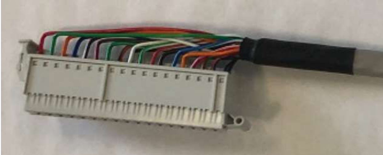
Figure 6. Conversion Module 18-Pin Connector on the 5069 Side
