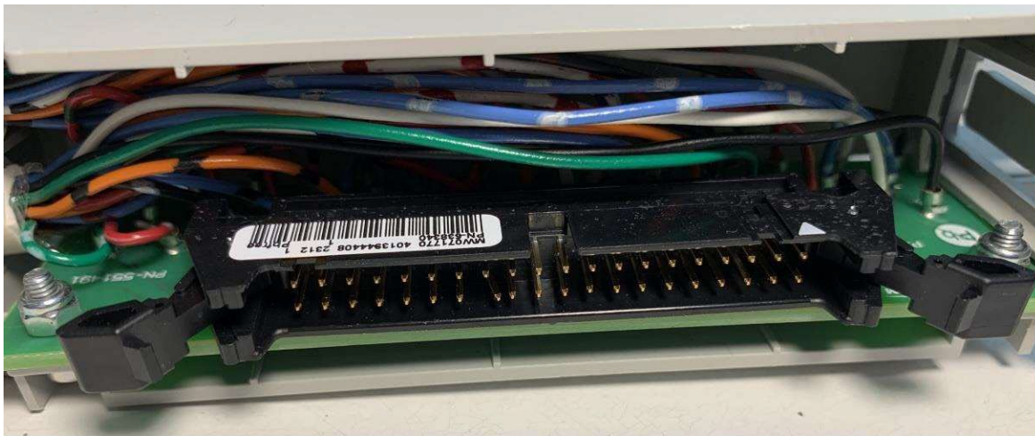
Figure 5. Conversion Module 40-Pin Field Connector on the 1746 Side
