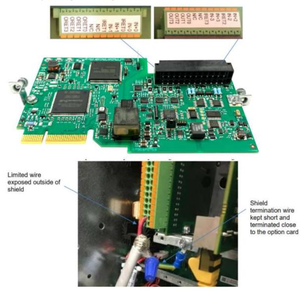
A given input on the card can be wired for any one of the following:
