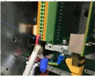
Shield termination wire kept short and terminated close to the option card
