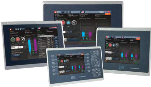
Figure 1. Operator interface panel HMIs, or graphic terminals, usually run a streamlined, embedded OS and dedicated software program with direct integration into the PLC or DCS being used. They're controlled via a touch interface or keys or push buttons on the panel itself.
