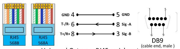
Universal Gateway RJ45 serial port to Siemens S7-200 DB9 RS485
