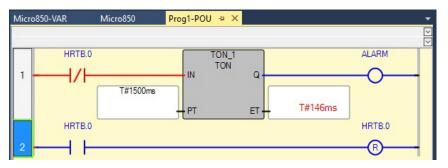
As with the other two examples the ladder logic is fundamentally the same in that the tag "HRTB" being "0" enables the timer and when it changes to "1" the timer is disabled and the bit "HRTB.0" resets it to "0". If the Gateway does not send a "1" to "HRTB" the time will eventually expire enabling the bit "ALARM".
