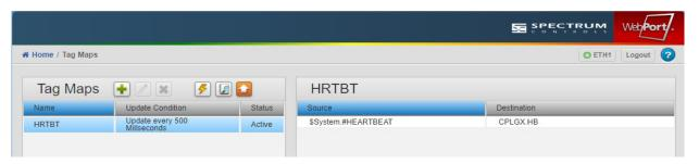
In the Logix example, a CompactLogix is configured with a tag labeled "HB" which is being updated every 500ms using the Heartbeat tag.
