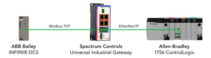
Challenge: Interfacing a Bailey® INFI90® DCS to a Rockwell Automation® ControlLogix® as part of a major plant upgrade with multiple stages.
