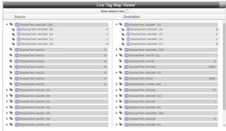
3. To view array values, click on the arrow associated with the array. The values appear on an indented, drop-down list in the column:
