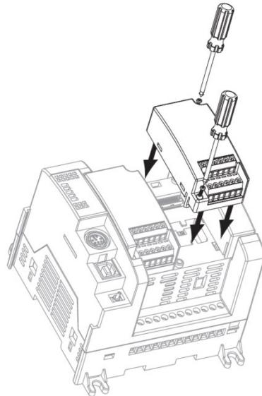
2. Snap the module into the module bay.
