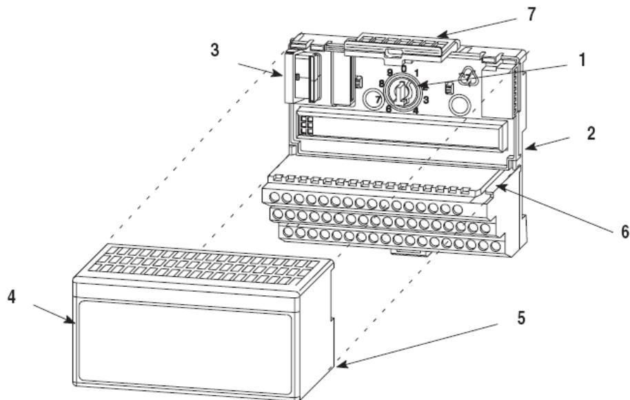
2. Make certain the FlexBus connector (3) is pushed all the way to the left to connect with the neighboring terminal base/adapter. **You cannot install the module unless the connector is fully extended.**
