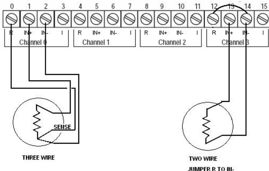
**Figure 2-3. Thermocouple Wiring Diagram**
