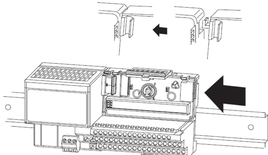
Slide the terminal base unit over tight against the adapter.
