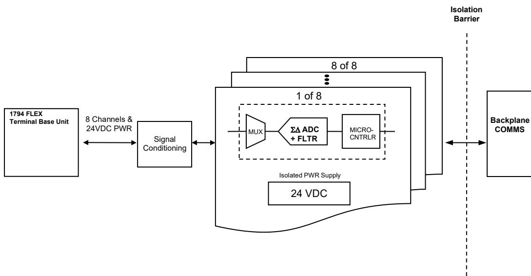
The module is designed to support up to 8 isolated channels of RTD, resistance, voltage, current, or thermocouple.
