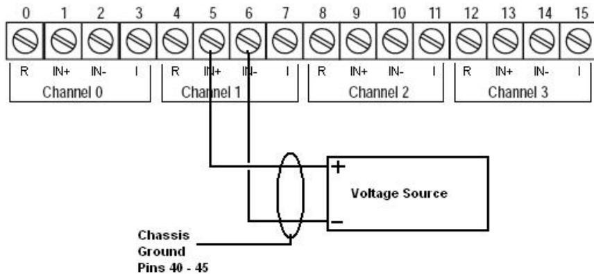
**Figure 2-5. Current Wiring Diagram**
