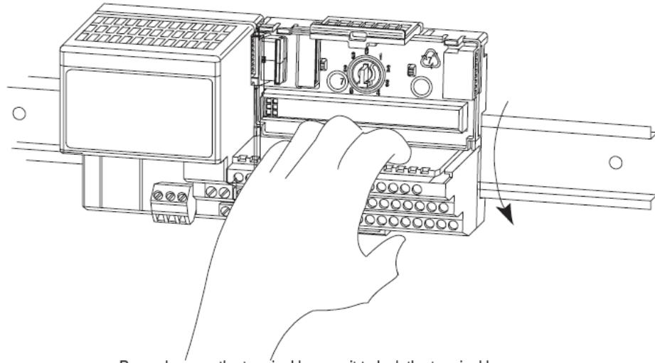
Press down on the terminal base unit to lock the terminal base on the DIN rail. If the terminal base does not lock into place, use a screwdriver or similar device to open the locking tab, press down on the terminal base until flush with the DIN rail and release the locking tab to lock the base in place.
