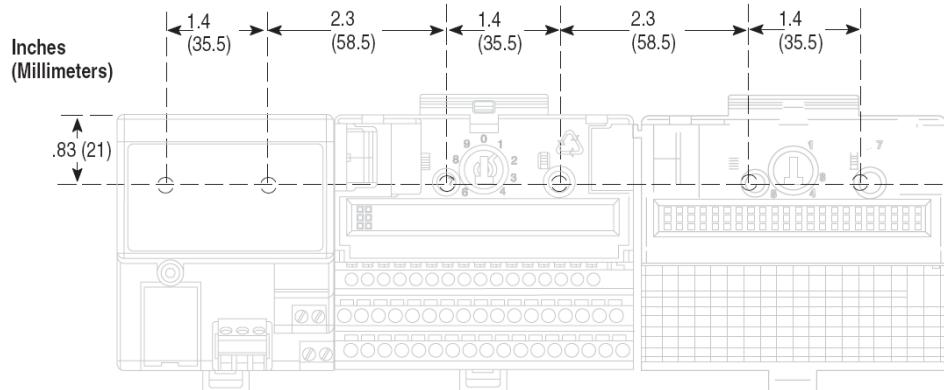
2. Drill the necessary holes for the #6 self-tapping mounting screws.
