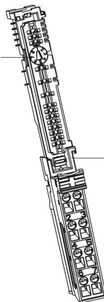
Be sure the DIN-rail locking screw is in the horizontal position.
