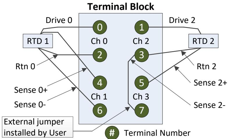
**Figure 2-7. System Configuration 4 (3-Wire and 4-Wire are Interchangeable)**
