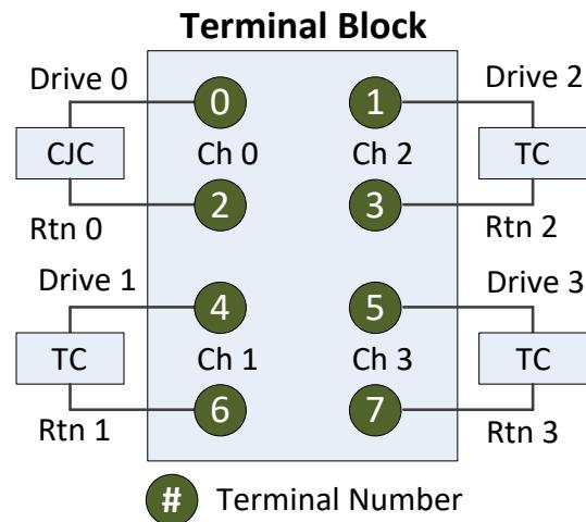
**Figure 2-15. System Configuration 12 All Current or Voltage**
