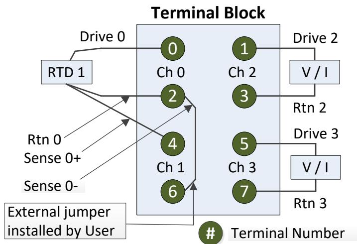
**Figure 2-10. System Configuration 7 (4-Wire RTD with Thermocouple)**
