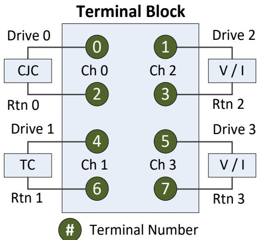
**Figure 2-13. System Configuration 10 Thermocouple with Voltage or Current**
