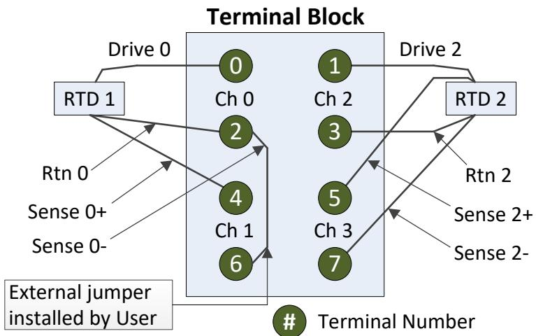
**Figure 2-8. System Configuration 5 (4-Wire RTD with Current or Voltage)**
