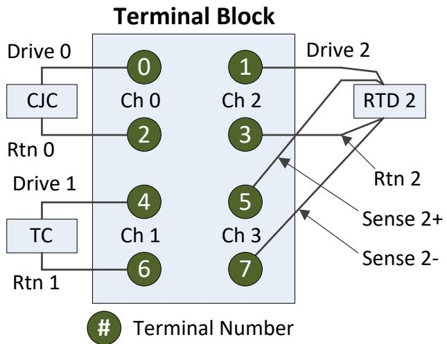
**Figure 2-11. System Configuration 8 (3-Wire RTD with Thermocouple)**
