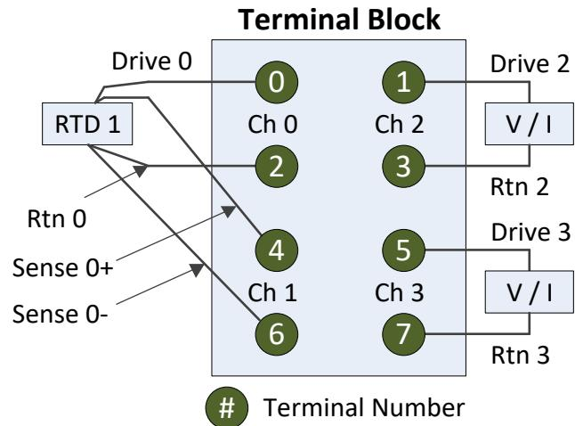
**Figure 2-9. System Configuration 6 (3-Wire RTD with Current or Voltage)**
