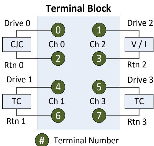
**Figure 2-14. System Configuration 11 All Thermocouples**
