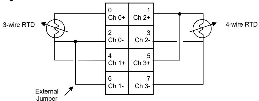
When measuring a 3-wire RTD, you **must** make an electrical short at the terminal block as shown below (see external jumper connection above):
