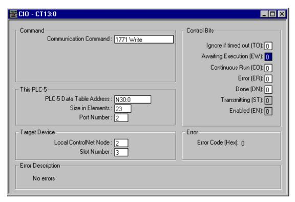
In this example, we have chosen the basic Module Configuration data size of 23 words. The data in the source Data File (N30:0 through N30:22) is entered by the user according to the 1771sc-IFE32 User Guide's Chapter 4.
