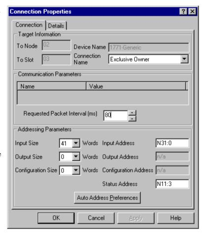
The Input Address chosen in the Connection Parameters dialog has already been chosen as the ControlNet Data Input file in the PLC-5. Input data from the module will be mapped into PLC-5 data file memory starting at that address.
