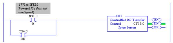
CIO instructions, like Block Transfers, use a control data block. The Control Block for a CIO is a "CT" data type, instead of a Block Transfer "BT" data type. The type of CIO which replaces a BTW is a "1771 Write".
