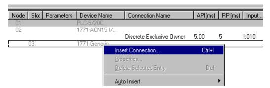
Enter the desired number of words into the Input Size field in the Connection Properties dialog.
