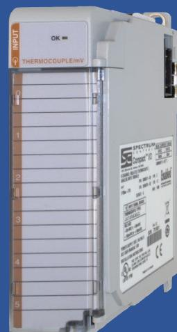
The 1769sc-IT6I/1769sc-IT6IK Input Modules provide full channel-to-channel isolated Thermocouple or millivolt input capability for noisy environments, in one I/O module. The 1769sc-IT6IK Input Module is conformally coated. The 1769sc-IT6I module can replace Thermocouple or Millivolt modules without compromising performance or price.
