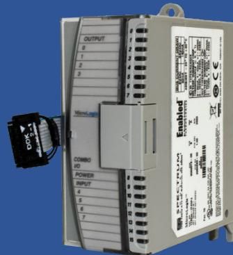
The 1762sc-IF4OF4 Combination Module provides full mixed analog capability in one I/O module. The 1762sc-IF4OF4 module can replace analog input, thermocouple, and analog output modules without compromising performance or price.
