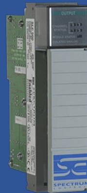
The 1746sc-INO4i and 1746sc-INO4vi Modules provide isolated analog output capability for noisy environments in individual I/O modules. The 1746sc-INO4i and 1746sc-INO4vi modules can replace analog output modules without compromising performance or price.
