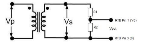
Let's say this is to be used on a 480V system. Since Vp=480Vac and Vs=24Vac, the nominal secondary output at a primary input of 480V would be (480/600)\*24=19.2Vac.
