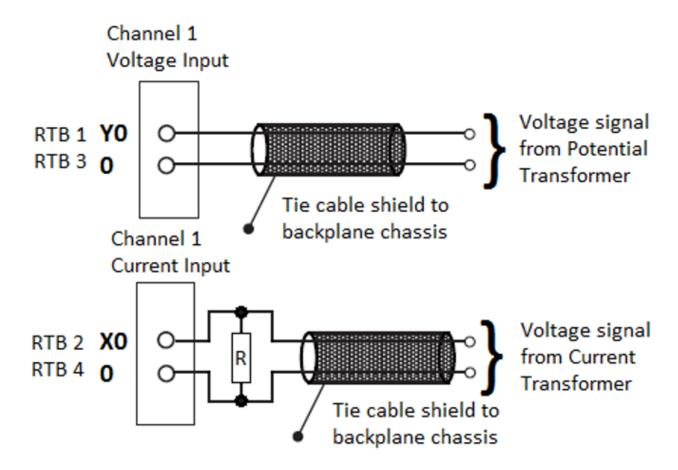
The 1756-RMS-SC module supports eight voltage/current input pairs connected individually to the module. Calculate the value of the load resistor (R=V/I) required for each current input by gathering up the following information:
