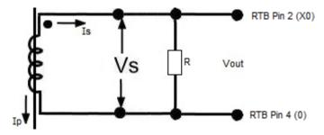
Since this CT has a ratio of 200:1, when the primary input is 200 amps, the secondary output will be 1 amp. The aim is to get Vout to be 5Vac when the secondary current Is is at 1 amp. R=V/A so 5 Volts/1 Amp means R should be 5 ohms. In the case of the CT we need to take into account the wattage of the resistor, so  $W=I^{2*}R=1*1*5=5$  watts. So this application needs a 5 watt, 5 ohm power resistor.
