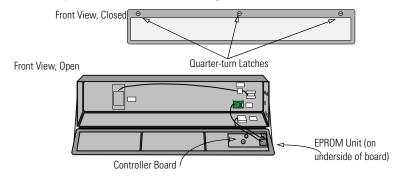
For the chip carrier type, on the underside of the controller board, firmly pull down on the end tabs of the EPROM and carefully pull it out of the socket.
