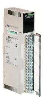
The 140 AUI 040 00sc provides Quantum Automation Series CPUs the capacity to handle a wide variety of analog input types. With 16 channels of input that can be configured in various combinations of RTD, thermocouple, current or voltage, this module is by far the most flexible analog input module available in the Quantum family of products.
